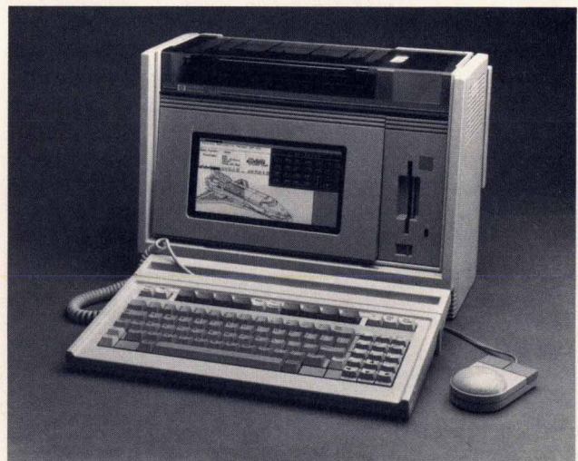
Fig. 2. HP's Integral Personal Computer 2 is a powerful multi-tasking computer system in a 25-lb transportable package. Designed for technical professionals, it features a built-in printer, display, disc drive, and HP-IB interface and the HP-UX operating system, HP's version of AT&T Bell Laboratories' UNIX ™ operating system.
