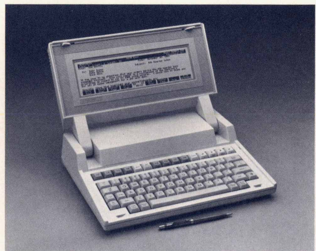
Fig. 4. The Portable is a 9-lb personal computer with built-in software for file management, spreadsheets, graphics, word processing, and data communications.
